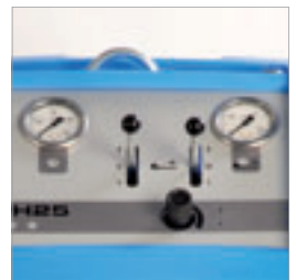
Pressure gauges for main and feed circuits
