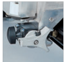
Simple saw head installation thanks to Y-carriage guide with fine adjustment
