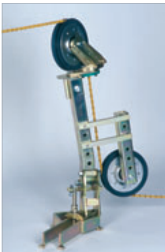
Universal support: Wire can be diverted in any direction
