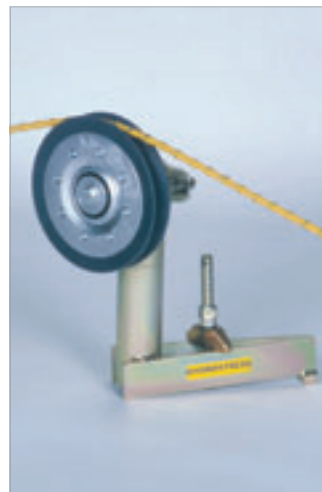
Diverter roll: Wire diversion with one adjustable axis
